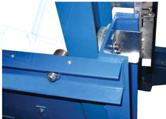
Figure 6. Lateral Guiding, 4 bearings per frame.
